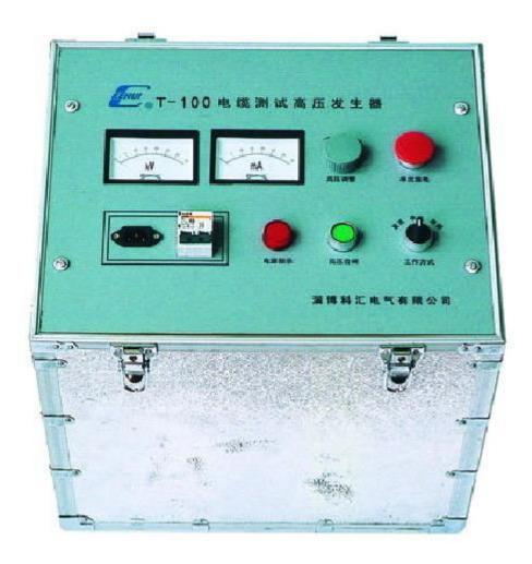
T-100 High Voltage Surge Generator is mainly used to discharge high voltage to the cable and burn down the faulty position, in conjunction with the Power Cable Fault Locator and Pinpointing Fault Locator, it can locate and pin-point cable faults like high resistance, low resistance and sheath faults.
