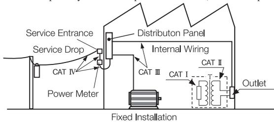
Higher-numbered categories correspond to electrical environments with greater momentary energy, so a measurement product designed for CAT III environments can endure greater momentary energy than one designed for CAT II.
