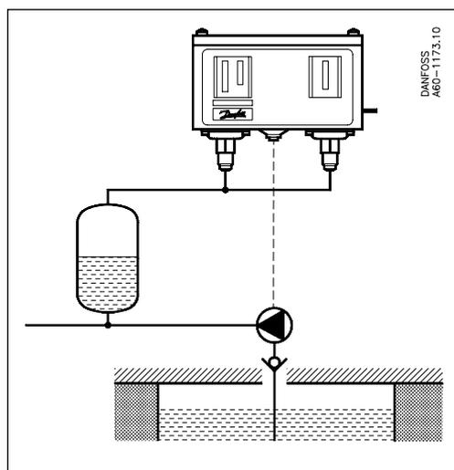
In a hydrophore system where water is pumped from a well or an open tank, both bellows are connected to a pressure outlet on the air side in the pump pressure line, if possible.
