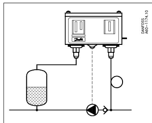
In a booster system receiving pressurized water the righthand bellows is connected - to the low pressure side of the pump for automatic start-up. - to the high pressure side of the pump for manual start-up.
