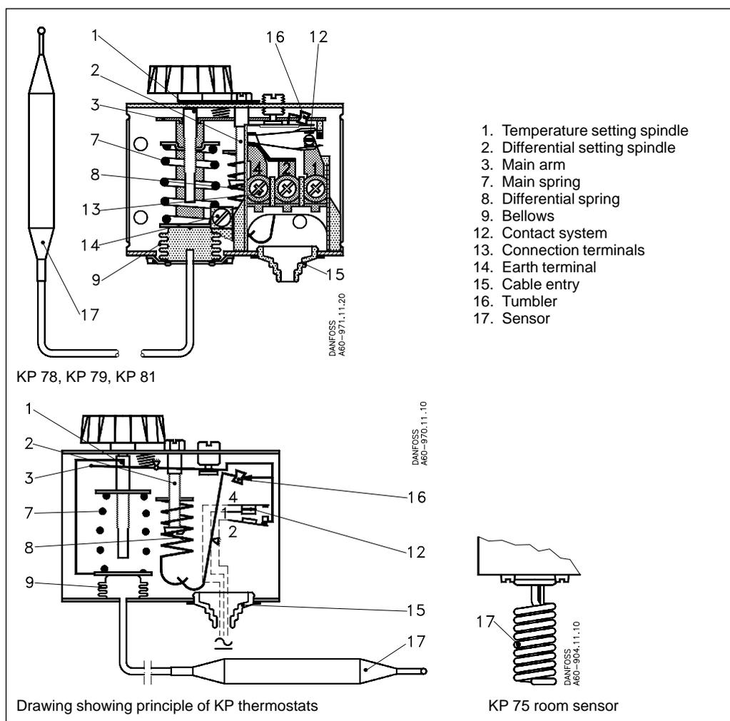
The contact system in KP thermostats has a snap function. This means that the bellows is active only when the cut-in or cut-out value is reached.
