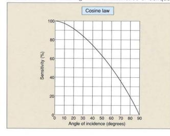
light on the illuminance meter much closer to this law. The following diagram shows the characteristics (typical response) of the 510 series illuminance meter which conforms to this new standard.
