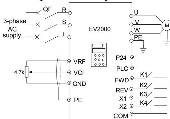
Fig. 5-58 Wiring of remote and local control
