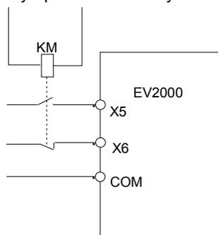
Fig. 5-41 Normally-open/close input
