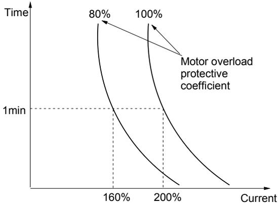
Fig. 5-71 Motor's overload protection coefficient
