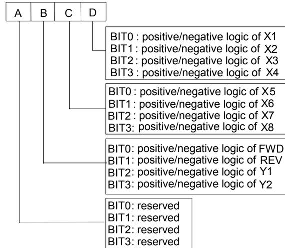
Fig. 5-51 terminal's positive and negative logic
