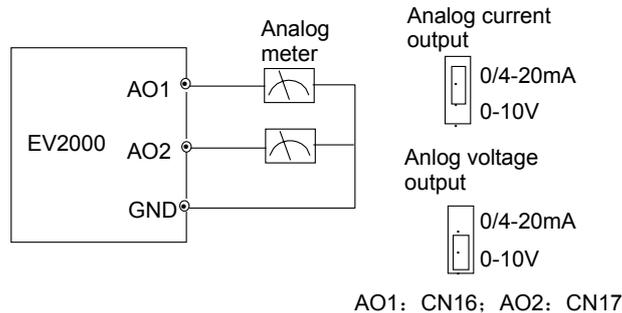
Fig. 3-16 Wiring analog output terminal
