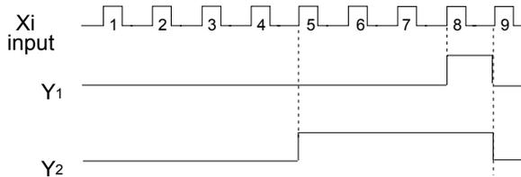
Fig. 5-50 Preset and specified pulse number
