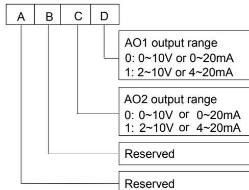
Fig. 5-49 analog output offset settings
