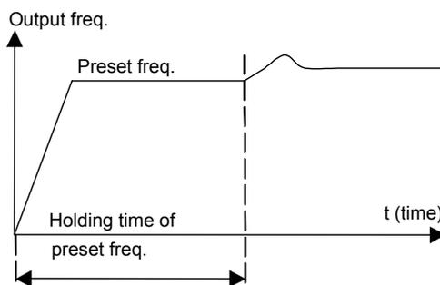
Fig. 5-36 Preset frequency of close-loop operation
