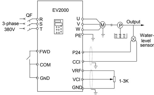
Fig. 5-29 Analog feedback control system with internal PI
