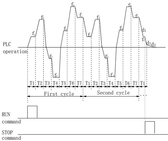
Fig. 5-25 Continuous operation of PLC
