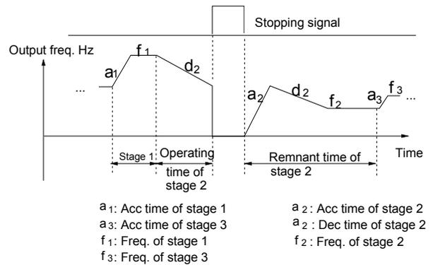
Fig. 5-27 PLC starting mode 2
