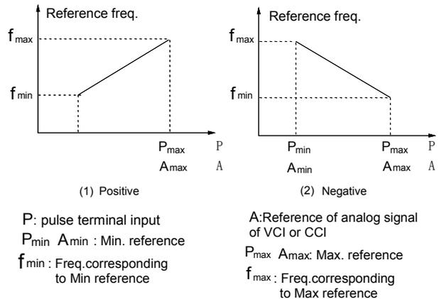
Fig. 5-8 Output frequency curve
