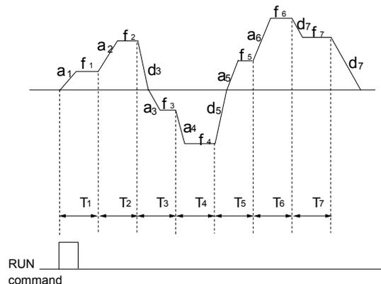
Fig. 5-23 Stopping mode after single cycle of PLC
