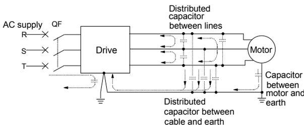
Fig. 3-42 Flowing path of leakage current
