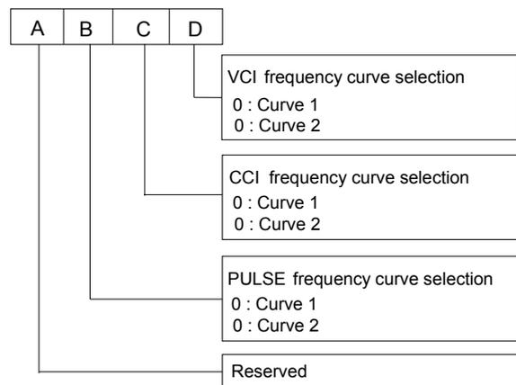
Fig. 5-9 Frequency curve selection
