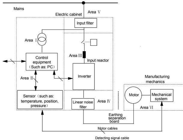
Fig. 3-43 Recommendation of Installation space
