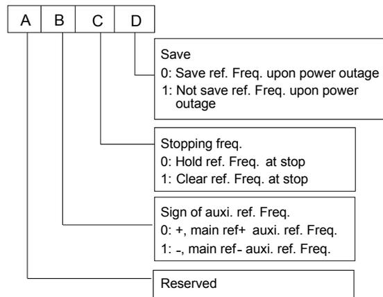
Fig. 5-63 Digital auxiliary reference frequency control
