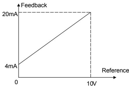
Fig. 5-32 Reference and feedback
