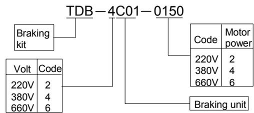
Fig. 2-6 Model of braking kit
