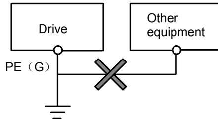
Fig. 3-40 Earthing diagram 4
