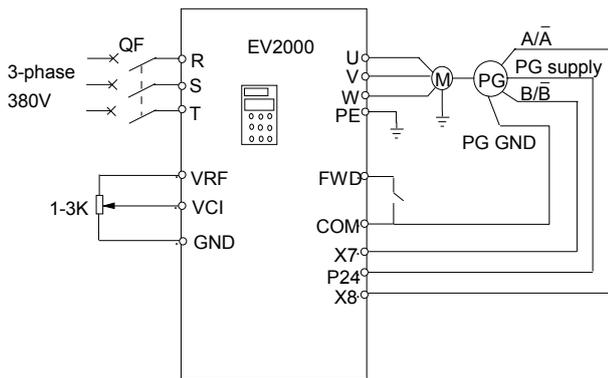
Fig. 5-30 Wiring of speed close-loop with PG
