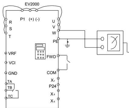
Fig. 7-1 Insulation test of drive
