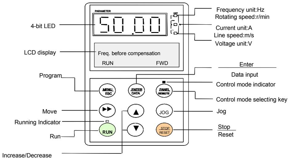
Fig. 4-2 Illustration of operation panel
