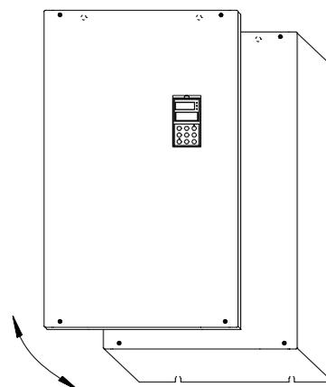
Fig. 3-6 Removing and mounting metal cover
