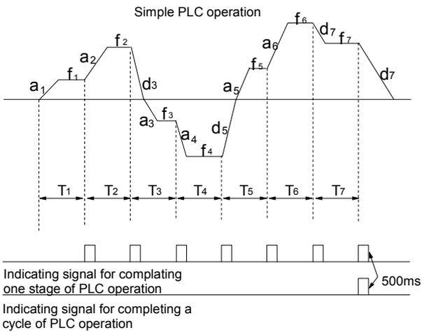
Fig. 5-21 Simple PLC operation
