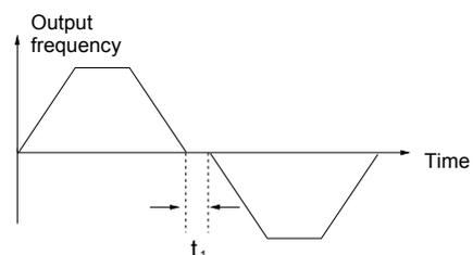
Fig. 5-17 Delay time from reverse running to forward running or from forward running to reverse running
