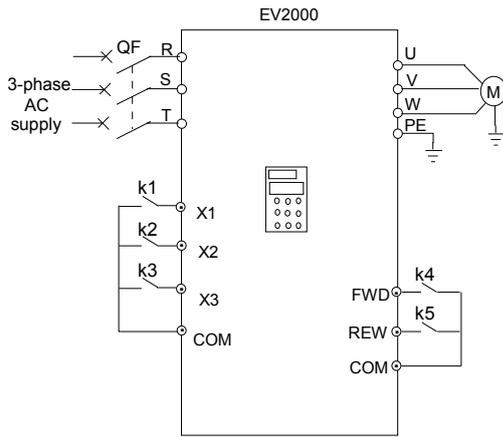
Fig. 5-40 Wiring for multi-speed operation
