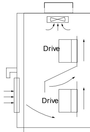
Fig. 3-3 Installation of several drives
