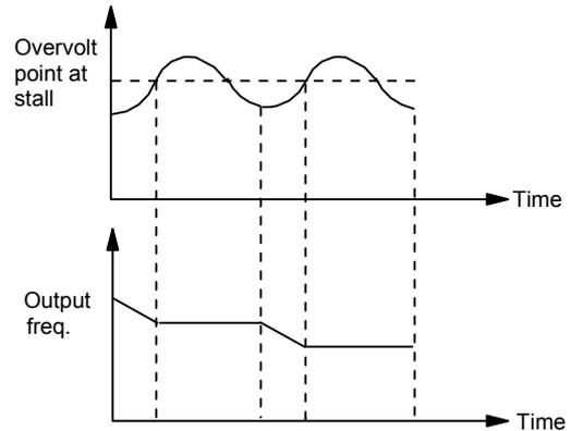
Fig. 5-72 Over-voltage at stall
