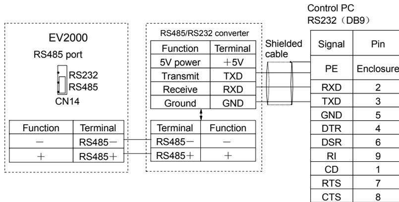
Fig. 3-18 RS485-(RS485/RS232)-RS232 communication cable
