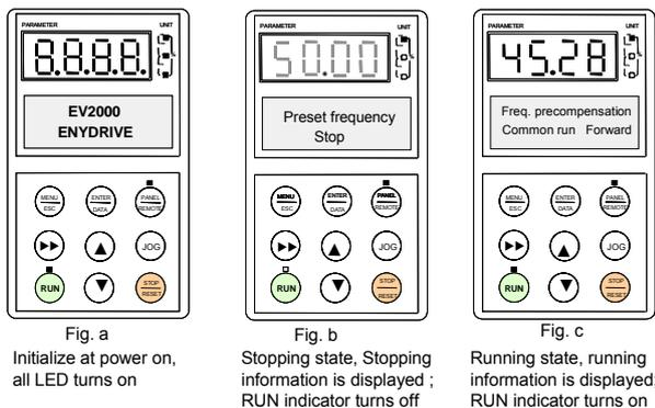
Fig. 4-4 Displayed during initialization, STOP, operation
