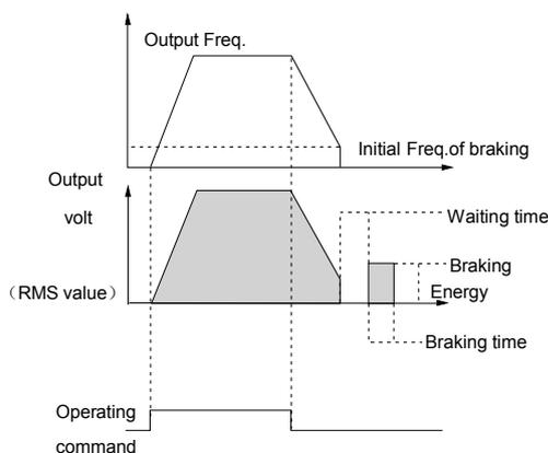
Fig. 5-16 Dec-to-stop + DC injection braking
