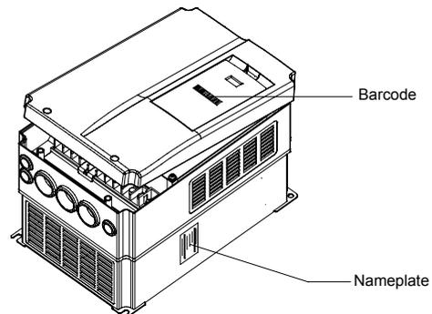
Fig. A-3 Locations of Nameplate and Barcode
