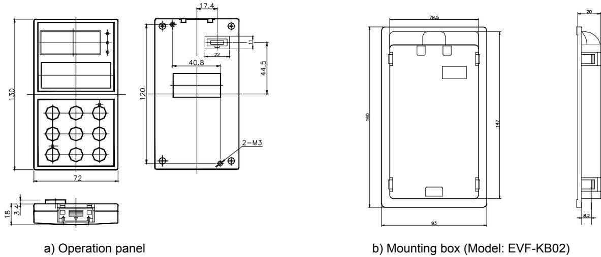
Fig. 2-4 Operation panel and mounting box
