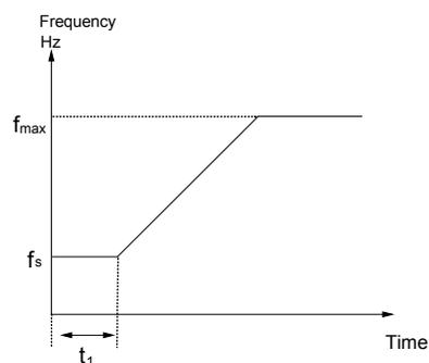
Fig. 5-12 Starting frequency and starting time
