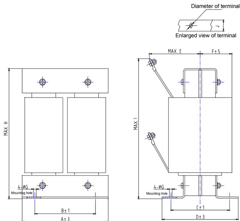
Fig. 2-3 Dimensions of DC reactor
