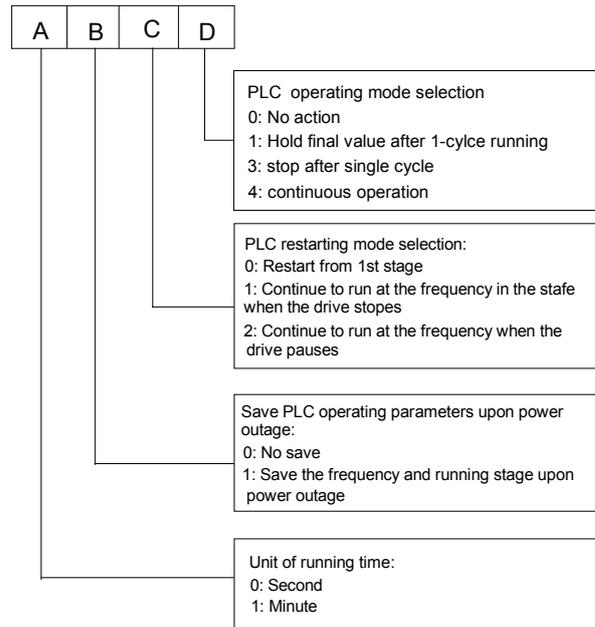
Fig. 5-22 Simple PLC operation mode
