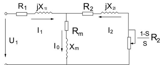
Fig. 5-70 Motor's equivalent circuit
