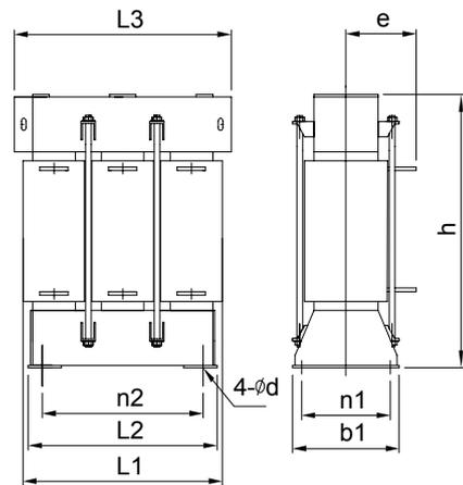
Fig. A-3 Outline of 3-PH AC input and output reactor (c)
