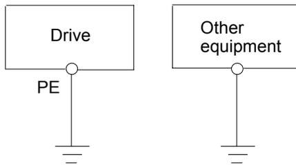
Fig. 3-37 Earthing diagram 1
