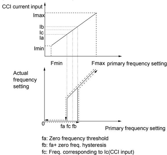
Fig. 5-67 Hysteresis of zero-frequency operation
