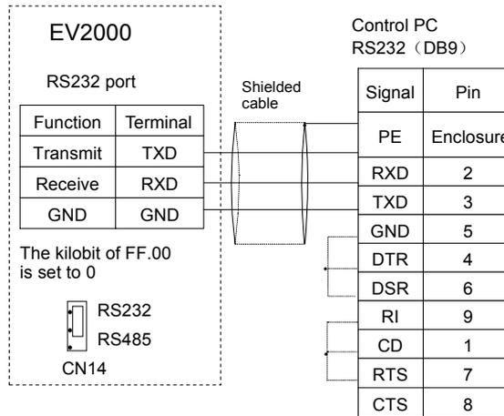
Fig. 3-17 RS232-RS232 communication cables
