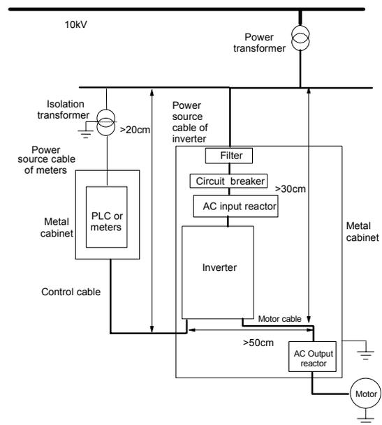
Fig. 3-44 Installation of the drive
