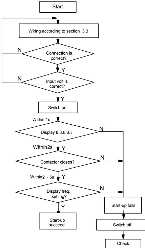
Fig. 4-8 Procedures of starting the drive for the first-time
