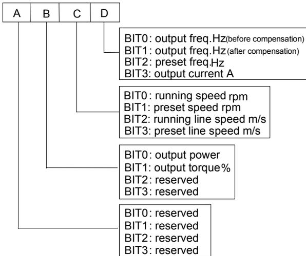
Fig. 5-52 LED displayed parameter group 1 in operation
