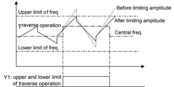
Fig. 5-46 Traverse operating amplitude control
