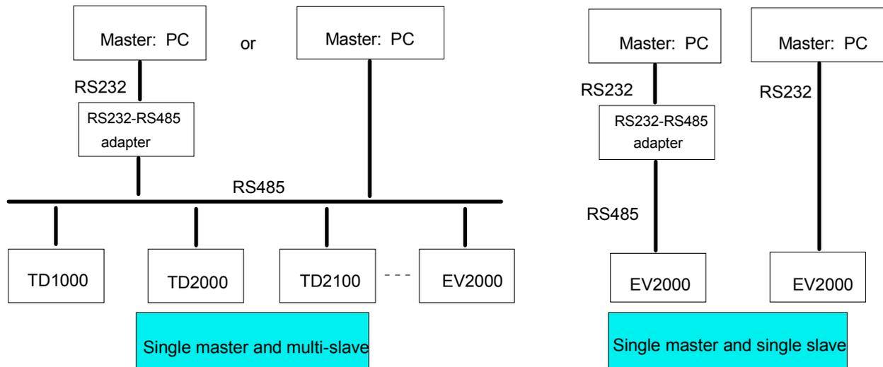
Fig. A-6 Networking diagram of drives
