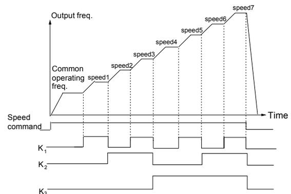
Fig. 5-39 Multi-step speed operation
