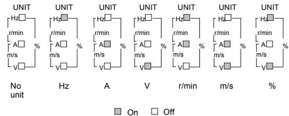
Fig. 4-3 Unit represented by combination of the indicators
