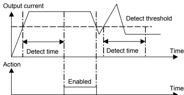
Fig. 5-74 Overload pre-alarm function
