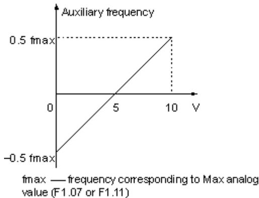
Fig. 5-61 VCI-5/CCI-5 as auxiliary ref. setting method
