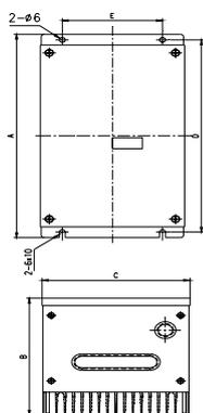
Fig. 2-8 Installation dimensions of braking kit
