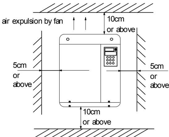
Fig. 3-1 Installation clearance (45kW or below)
