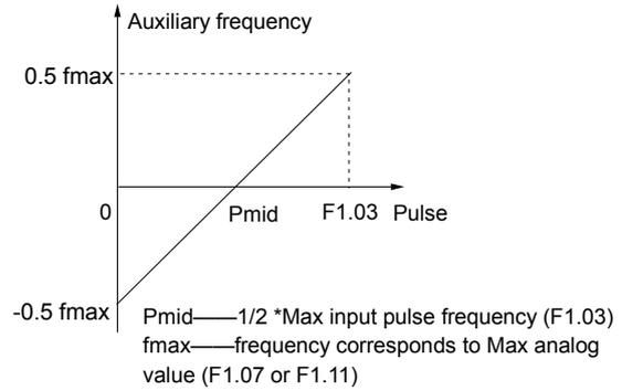
Fig. 5-62 PULSE-0.5×F1.03 as auxiliary ref. setting method
