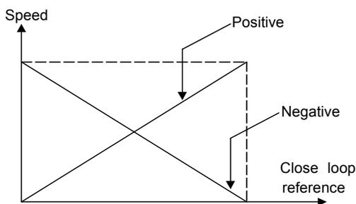
Fig. 5-33 Close-loop control characteristic
