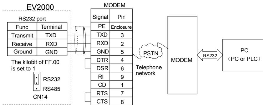
Fig. 3-19 Wiring of RS232-(MODEM-PSTN-MODEM)-RS232 communication
