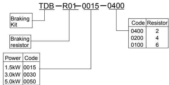
Fig. 2-7 Explanations of Model of braking resistor
