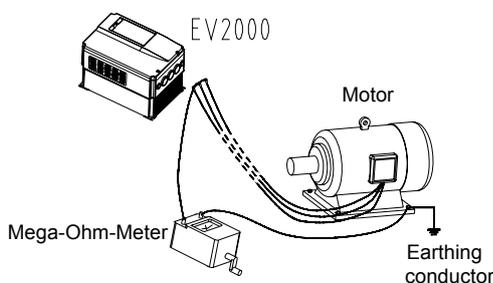
Fig. 1-1 Checking the insulation of motor
