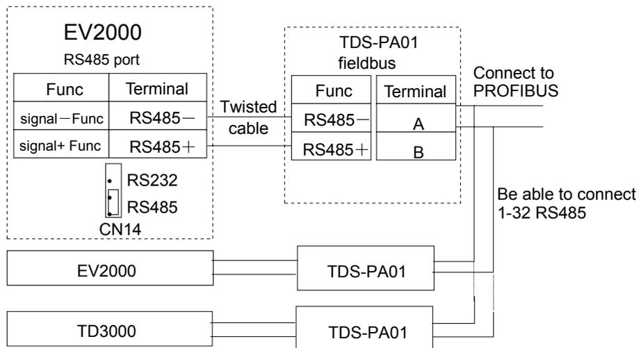
Fig. 3-20 Wire connections of RS485-(TDS-PA01)-PROFIBUS communication
