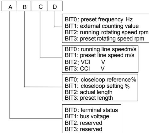
Fig. 5-55 Stopping parameters displayed by LED
