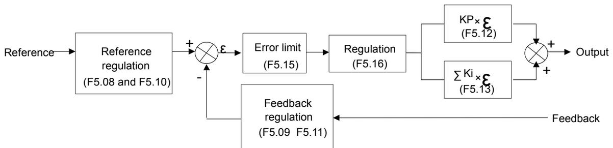
Fig. 5-31 PI block diagram
