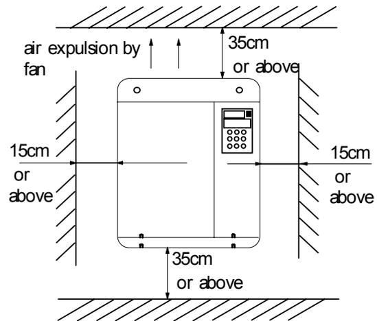
Fig. 3-2 Installation clearance(55kW or above)
