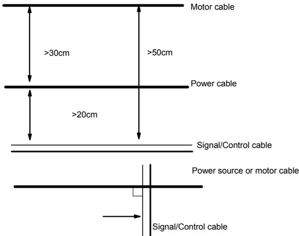
Fig. 3-34 Wire connections
