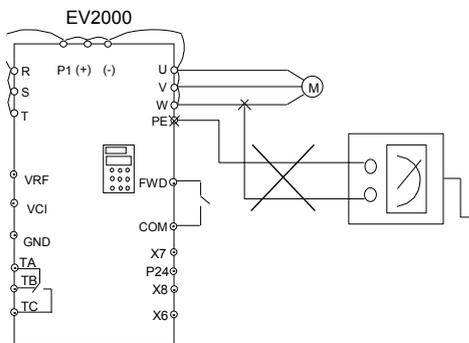
Fig. 7-2 Insulation test of motor
