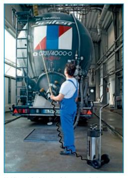
Mobile and flexible: the right partner for long distances. If larger distances have to be covered regularly when working with the sprayer, the TKS and TRK models offer significant advantages. The spiral hose (TKS) expands up to 5 m if requested. The use of the optional transport trolley enables a change of location noticeably easier.
